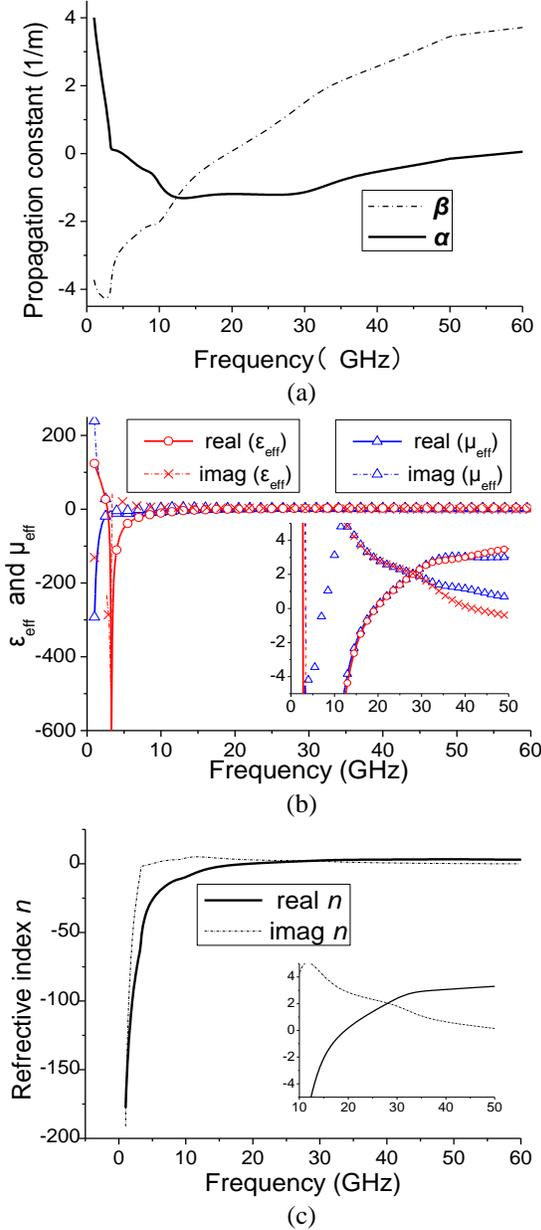
Fig. 3. (a) Extracted complex propagation constant  $\gamma(\alpha+j\beta)$  from measured two-port S-parameter. (b) Extracted effective permittivity  $\epsilon_{\text{eff}}$  (red) and effective permeability  $\mu_{\text{eff}}$  (blue) from measured two-port S-parameter. The inset shows the details near zero-Y-axis. (c) Extracted index of refraction  $n$  from measured two-port S-parameter. The inset shows the details near zero-Y-axis.
