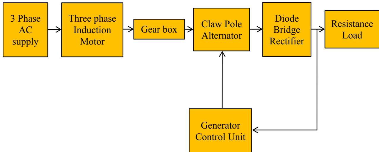
Fig. 11. Experimental set-up of the proposed alternator.
