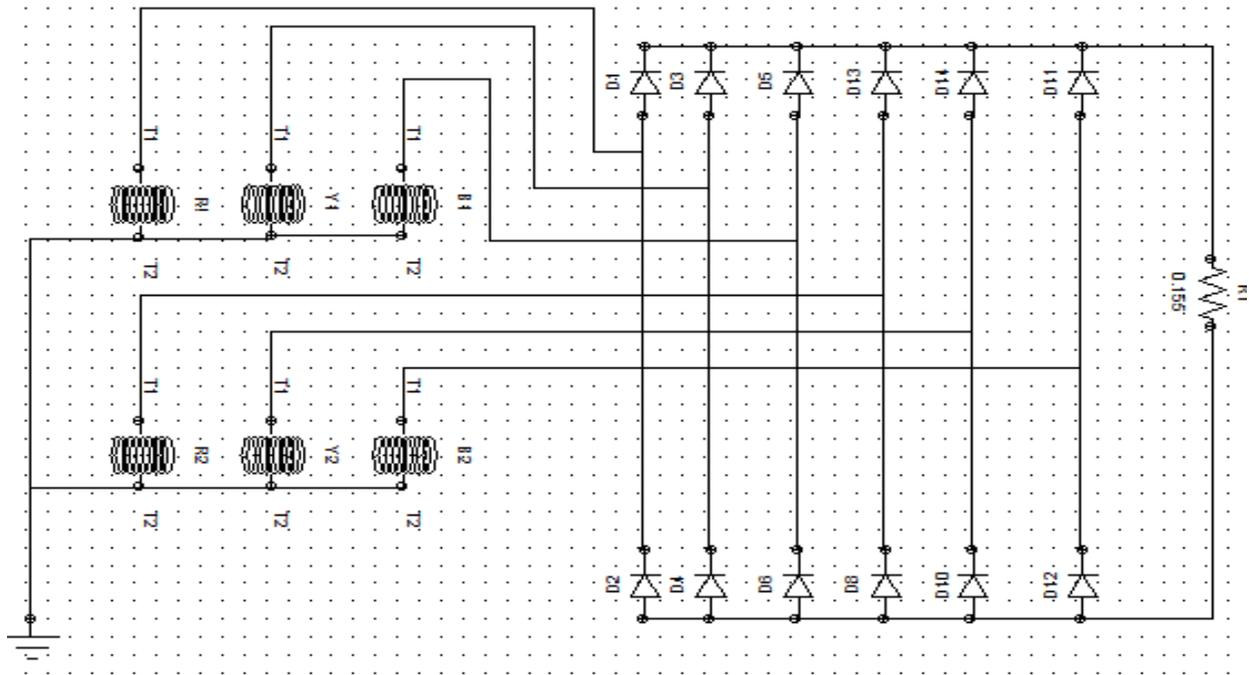
Fig. 8. Stator coil connected to external load.
