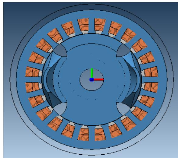
Fig. 4. 3D model of claw pole alternator.
