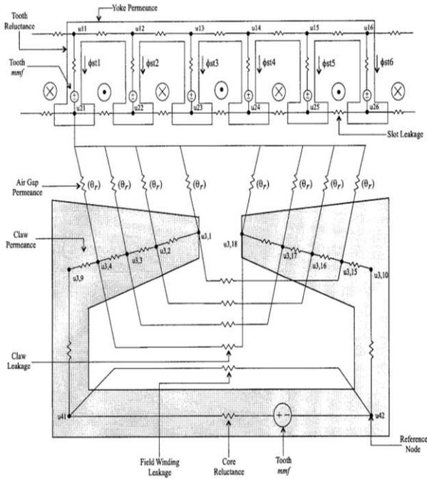
Fig. 2. Magnetic equivalent circuit of claw pole alternator.
