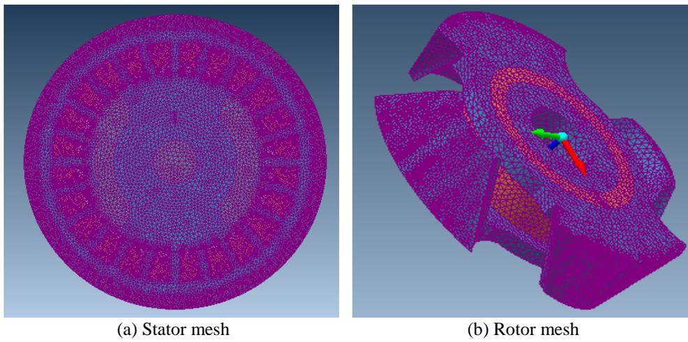
Fig. 6. Stator and rotor mesh generation.
