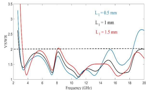
Fig. 3. VSWR of the antenna with different values of  $L_1$  when  $W_1$  is fixed at 0.8 mm.
