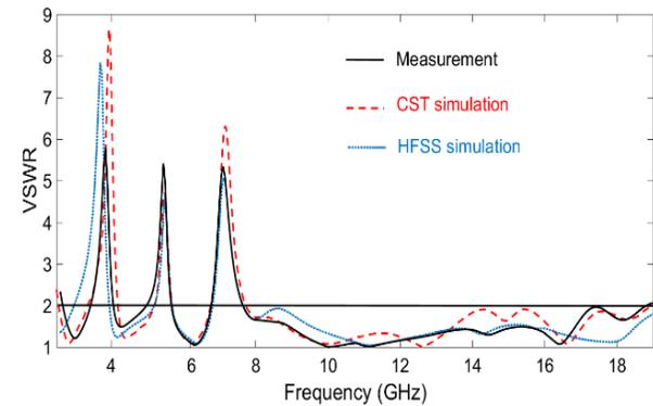
Fig. 6. Measured and simulated VSWR of proposed antenna.
