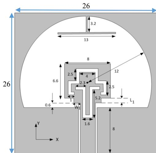
Fig. 1. Geometry of the proposed antenna (mm).
