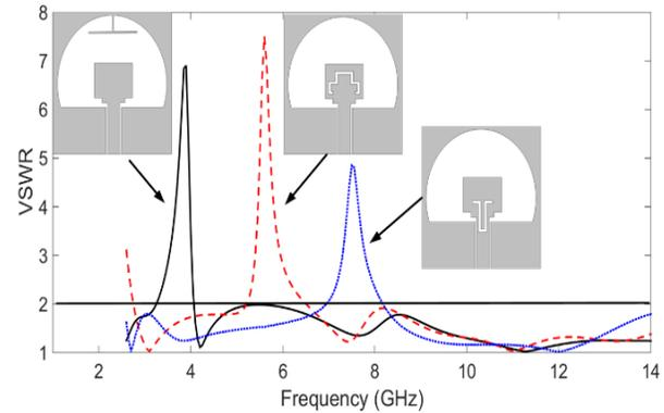
Fig. 5. VSWR of different single band notched antennas.
