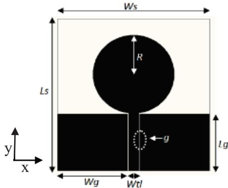
Fig. 3. Geometry of the proposed transparent UWB antenna.
