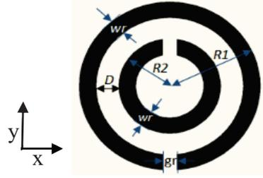
Fig. 1. Geometry of the split ring resonator.
