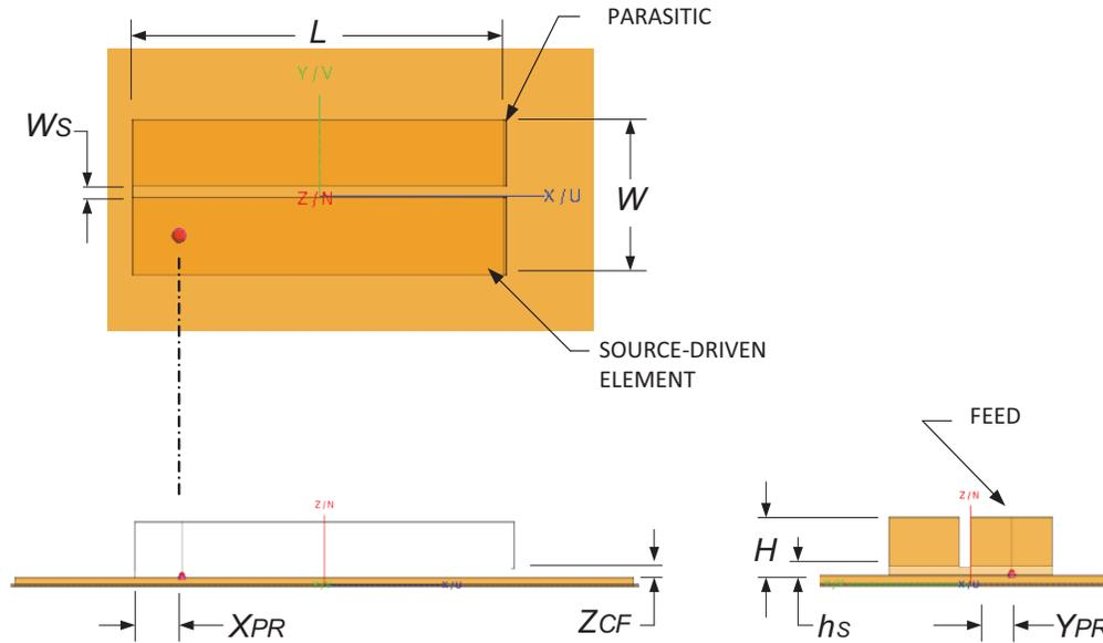
Fig. 1. Engineering perspective of multi-resonant planar inverted-F antenna.
