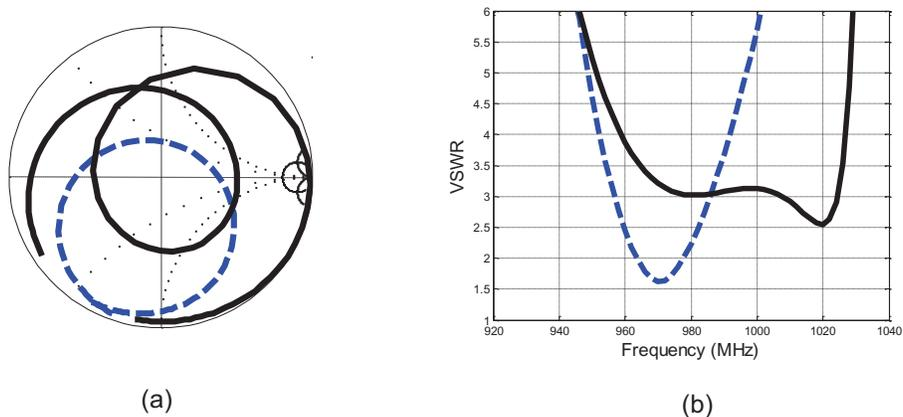
Fig. 2. (a) Normalized impedance and (b) VSWR responses for multi-resonant (solid) and single-resonant (dashed) planar inverted-F antennas with similar form-factors. The boundary condition for both simulations shown was a perfect-electrically-conducting (PEC) infinite ground plane.
