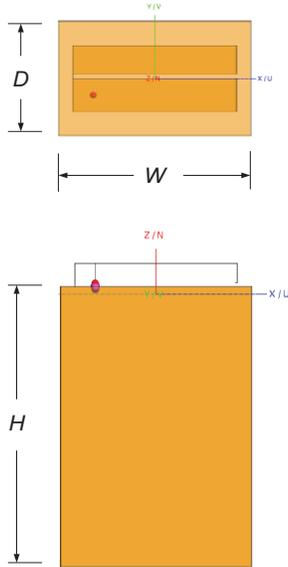
Fig. 3. CADFEKO rendering of double-resonant PIFA integrated to handheld device platform. The dimensions of the lossless chassis are approximately  $H=10\text{ cm}$ ,  $W=6.5\text{ cm}$  and  $D=4.0\text{ cm}$ .
