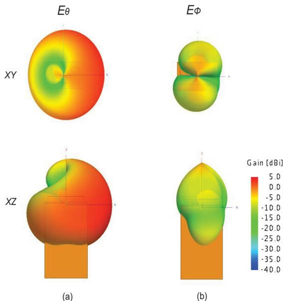
Fig. 6. POSTFEKO renderings of:(a)  $E_\theta$  and (b)  $E_\phi$  radiation patterns for the multi-resonant PIFA mounted on a handheld chassis.
