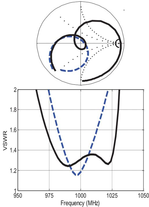
Fig. 5. (a) Normalized impedance and (b) VSWR for the double resonant (solid) and single-resonant (dashed) PIFA integrated to handheld device (shown in Fig. 3).
