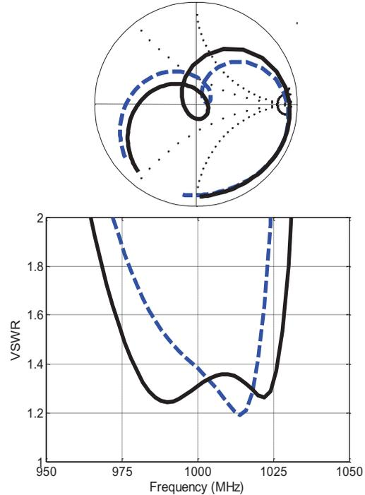
Fig. 4. Impedance responses for ‘untuned’ (dashed) and ‘tuned’ (solid) double-resonant PIFAs integrated to a handheld device (shown in Fig. 3). The observed results are the double-tuning is maintained but with adjustments to the parameters of the coupling slot, an increase in 2:1 VSWR impedance bandwidth of  $\Delta B \approx 25\%$  may be obtained.
