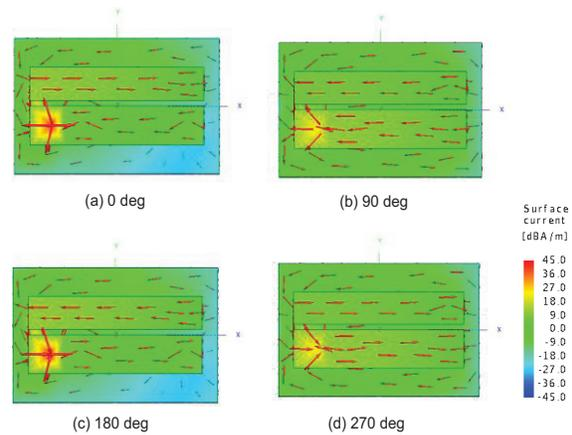
Fig. 7. Surface current distributions on handheld PIFA geometry for  $\omega t = [0^\circ, 90^\circ, 180^\circ, 270^\circ]$ .
