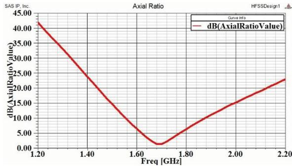
Fig. 9. Axial ratio (AR) diagram versus frequency of the antenna.
