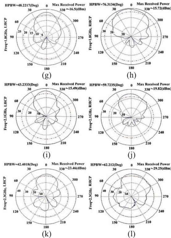
Fig. 12. Normalized measured radiation pattern results at six frequencies of Fig. 11; left column: LHCP, right column: RHCP.
