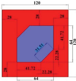
Fig. 4. Patch characteristics and dimensions (in mm).
