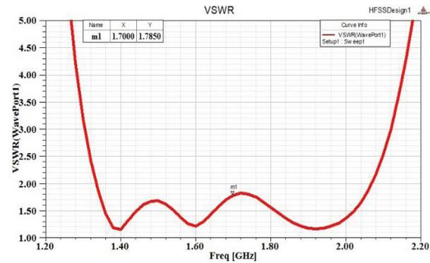
Fig. 6. VSWR diagram of the antenna.
