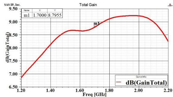
Fig. 8. Gain diagram versus frequency of the antenna.
