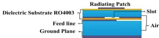
Fig. 1. Side view of aperture coupled microstrip antenna.
