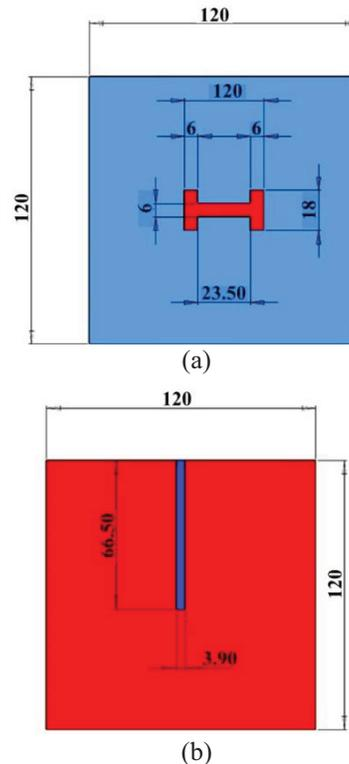
Fig. 3. (a) Feeding network and (b) slot (dimensions in mm).
