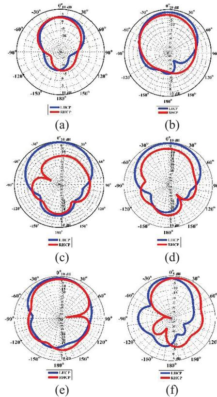
Fig. 11. Simulated radiation pattern results at: (a) 1.3 GHz, (b) 1.5 GHz, (c) 1.7 GHz, (d) 1.8 GHz, (e) 2.1 GHz, and (f) 2.3 GHz.
