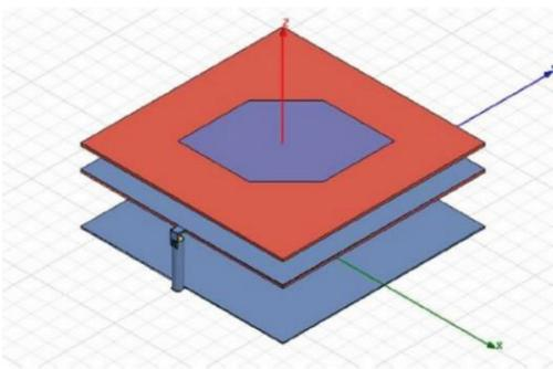
Fig. 5. Illustration of aperture coupled microstrip antenna.
