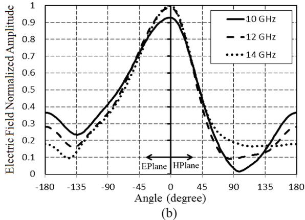
Fig. 2. Radiation characteristics of double ridged horn antenna: (a) VSWR, (b) normalized amplitude of electric field radiation patterns, E and H-plane.
