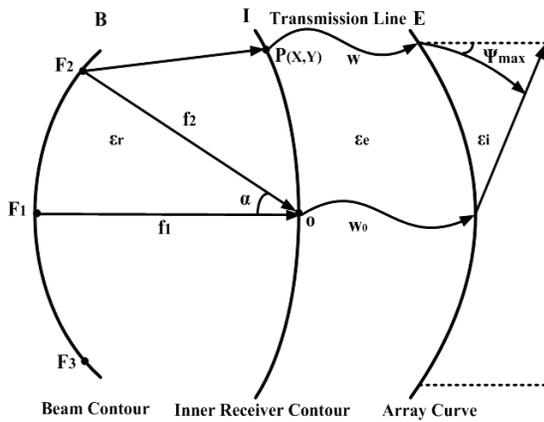
Fig. 1. Trifocal Rotman lens structure for conformal arrays.
