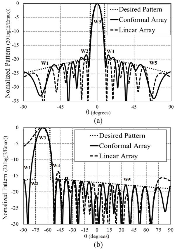
Fig. 4. Optimized radiation patterns: (a) zero scan angle ( $w_1=w_5=0.4$ ,  $w_2=w_4=2.2$  and  $w_3=1.8$ ), (b)  $-65^\circ$  scan angle ( $w_1=0.8$ ,  $w_2=1.8$ ,  $w_3=3.4$ ,  $w_4=2.8$  and  $w_5=1.6$ ).
