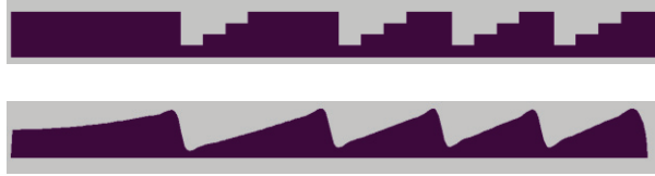
Fig. 1. Schematic profile of a conventional FZPA with 5 zones and 4 steps and schematic profile of the proposed FZPA.
