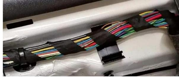
Fig. 1. Handmade cable bundles under car window.
