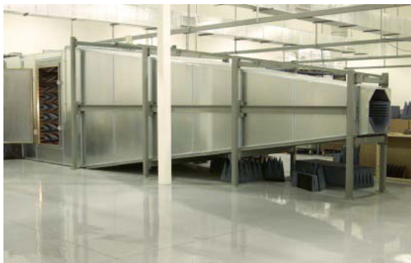
Fig. 1. A typical tapered anechoic chamber.
