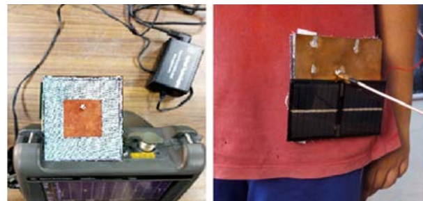
Fig. 10. Proposed wearable antenna measurement setup.
