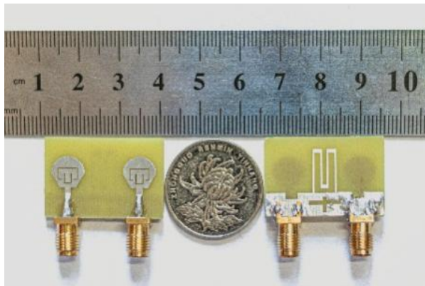
Fig. 9. Fabricated prototype of proposed two-port MIMO antenna.
