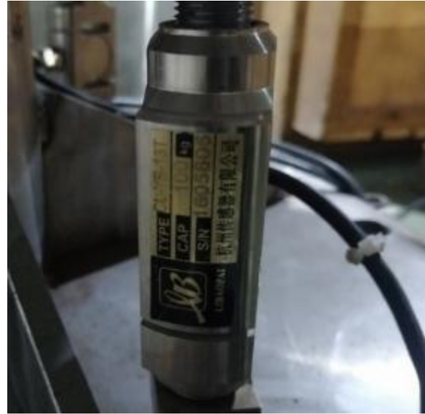
Fig. 2. CL-YB-13T/100kg force measuring sensor.
