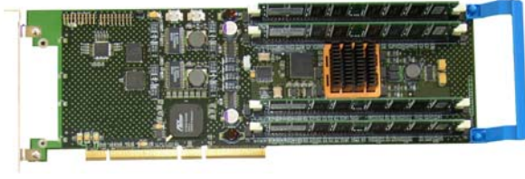
Fig. 1. The FDTD hardware accelerator. This FPGA-based board provides the platform for the acceleration architecture. It includes the largest FPGA on the market and supports up to 16 GB DDR SDRAM. This platform has demonstrated performance comparable to 100-node PC clusters.
