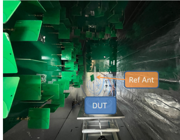
Fig. 7. The TRP measurement scenario in an RC.
