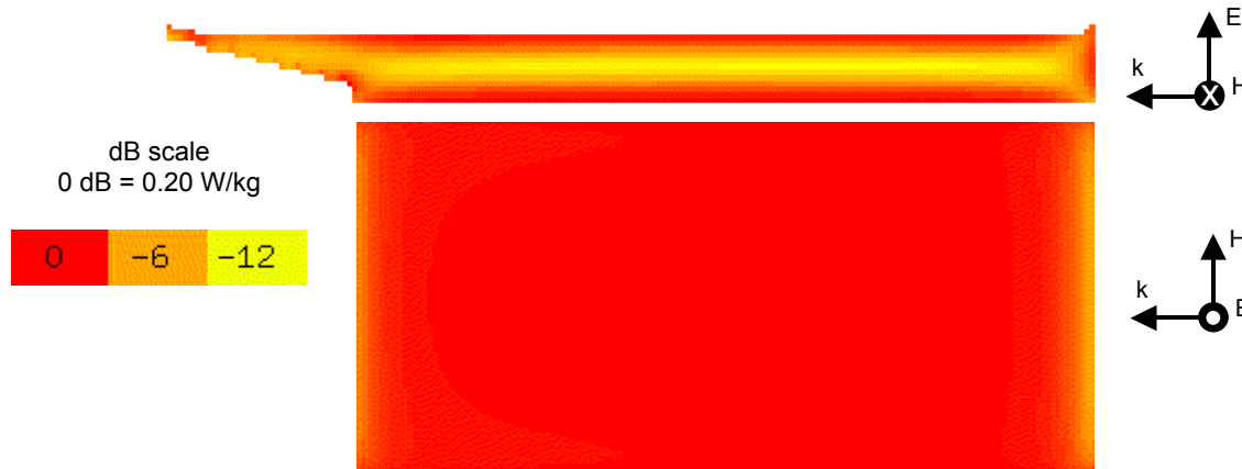
Figure 5. SAR profile in the RPMI medium. top: Slice through the middle (note the medium in the neck of the flask on the left). bottom: Bottom layer where cell culture resides.
