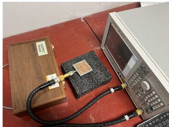
Fig. 11. The measurement of the proposed filtering antenna.
