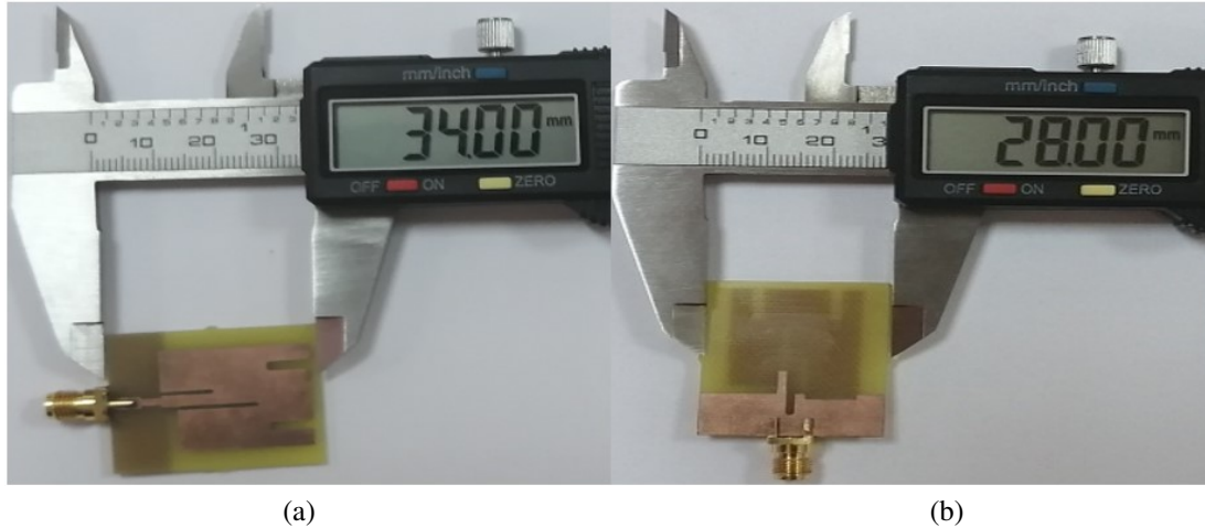
Fig. 6. Fabricated prototype of the proposed CPPMA: (a) front view and (b) back view.
