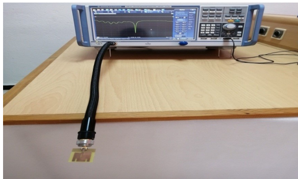
Fig. 7. Reflection coefficient setup measurement of the proposed CPPMA.
