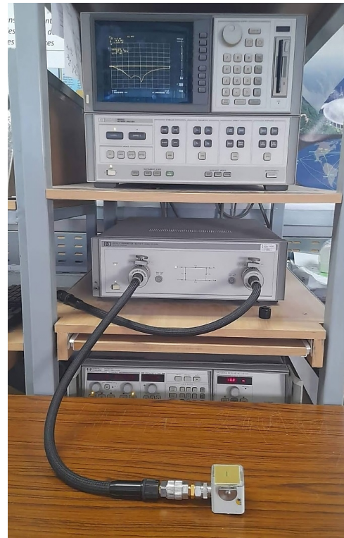
Fig. 12. Photograph of measurement set-up: Reflection coefficient measurement.
