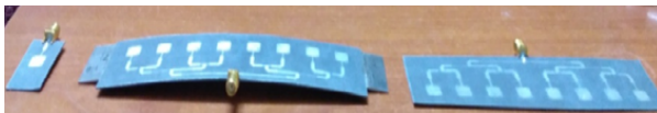
Fig. 15. Single-element proposed planar microstrip antenna array and conformal microstrip antenna array fabrication.
