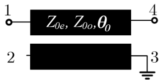
Fig. 2. Schematic of the proposed 2-port band stop filter based on parallel-coupled lines.
