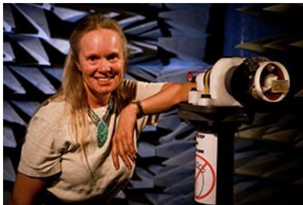
Fig. 8. Professor Furse in an anechoic chamber measuring an antenna.
