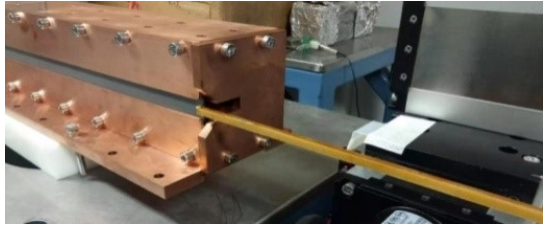
Fig. 9. Point coil for measuring the end field.
