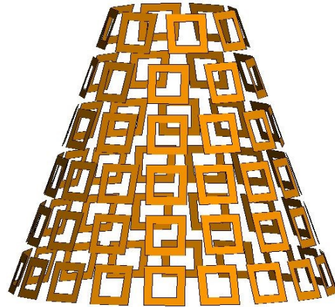
Fig. 4. Geometry of the square ring FSS conical radome.
