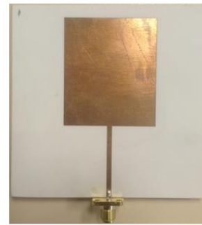
Fig. 3. Photograph of the fabricated wide-band monopole antenna.
