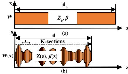
Fig. 1. (a) UTL and (b) NTL with its subdivision into  $K$  uniform sections.
