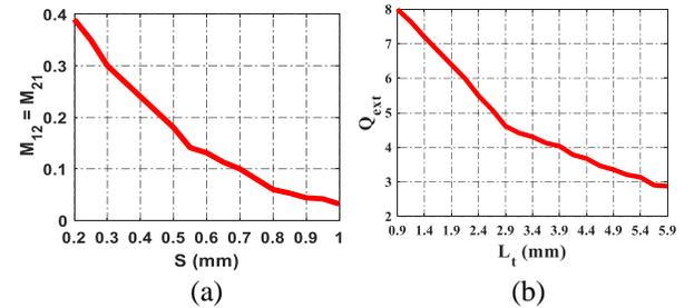
Fig. 2. Relation between (a)  $M_{12}$  and  $S$  and (b)  $Q_{ext}$  and  $L_t$ .
