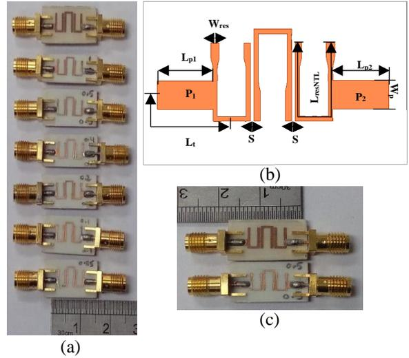
Fig. 5. (a) Fabricated prototypes of 6.55 GHz NTL HPBF at six different  $\Delta f$ s, (b) configuration of the proposed 6.55 GHz NTL HPBF at  $\Delta f = 0.5$ , and (c) fabricated prototypes of 6.55 GHz UTL and NTL HPBF.
