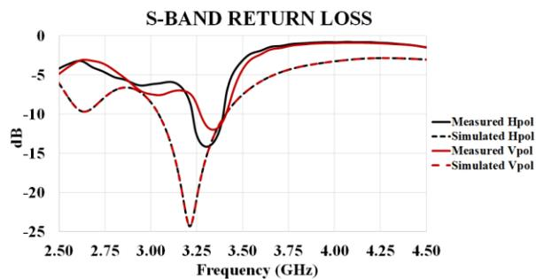
Fig. 4. Return loss comparison at S-band ports.
