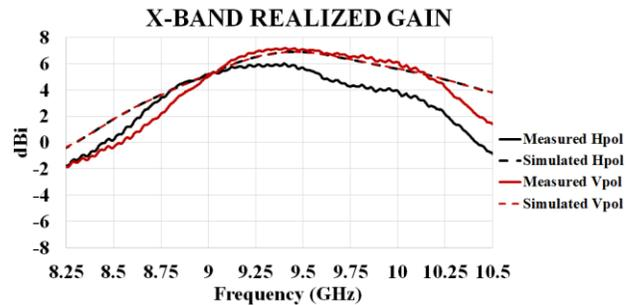
Fig. 7. Realized gain comparison at X-band ports.
