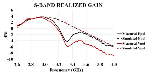
Fig. 5. Realized gain comparison at S-band ports.
