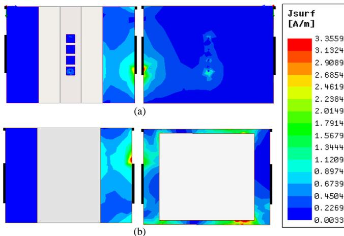
Fig. 4. Surface current distributions (port 2 excited), patches on the left and ground plane on the right: (a) with EBG and (b) without EBG.
