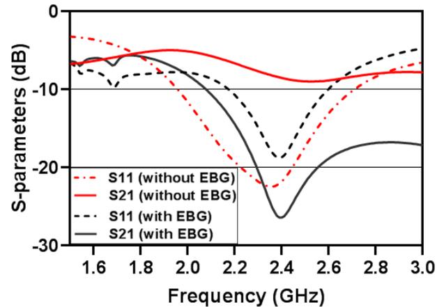
Fig. 2. Simulated S-parameters with and without EBG.
