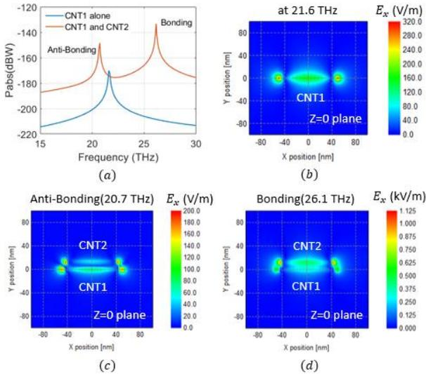
Fig. 2. (a) Absorbed power spectrums: CNT1 alone Vs CNT Dimer with 20a dimer gap (calculated by in-house algorithm). (b) Magnitude of  $E_x$  near-field component for CNT1 at 21.6 THz. (c) CNT-dimer at 20.7 THz (Anti-bonding mode). (d) CNT-dimer at 26.1 THz (Bonding mode). (Simulated in FEKO 3D MOM solver [6]).
