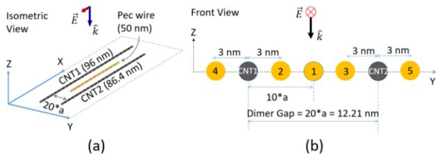
Fig. 1. (a) Asymmetric CNT dimer along with a PEC nano-wire placed at the center of the dimer gap excited with an  $x$ -polarized normally incident plane wave, and (b) schematic view of five different  $y$ -locations of the PEC nano-wire on the same plane as the CNT dimer.
