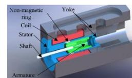
Fig. 1. Geometry structure definition of LPS three-dimensional simulation model.
