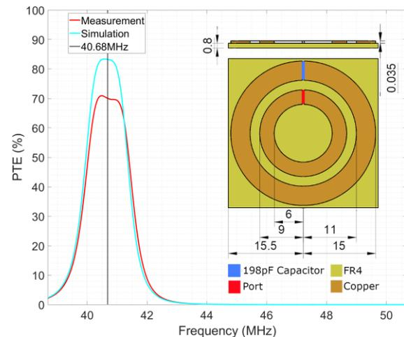
Fig. 1. Simulated and measured PTE versus frequency.
