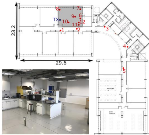
Fig. 5. Blueprint of the measurement site with the transmitter and receiver points. The gray area on the top is shown in detail on the inferior part.
