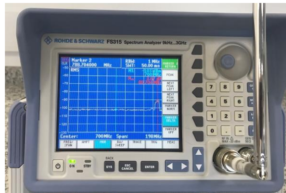
Fig. 4. Spectrum analyzer used as receiver, with telescopic antenna, measuring the environment noise floor.
