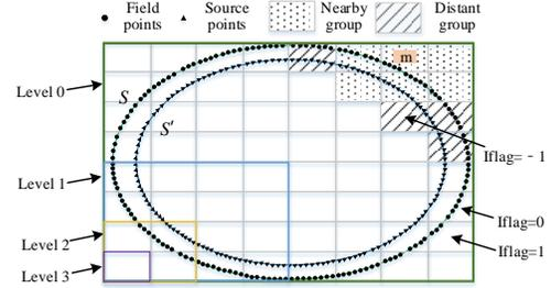
Fig. 2 Configuration for MLFMA based near-field computation.
