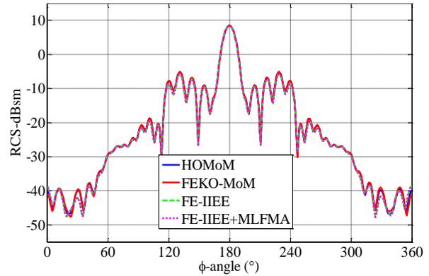
Fig. 6. Bistatic RCS results of the low scattering carrier at 3.0 GHz in the  $xoy$ -plane calculated by the proposed method and MoM.
