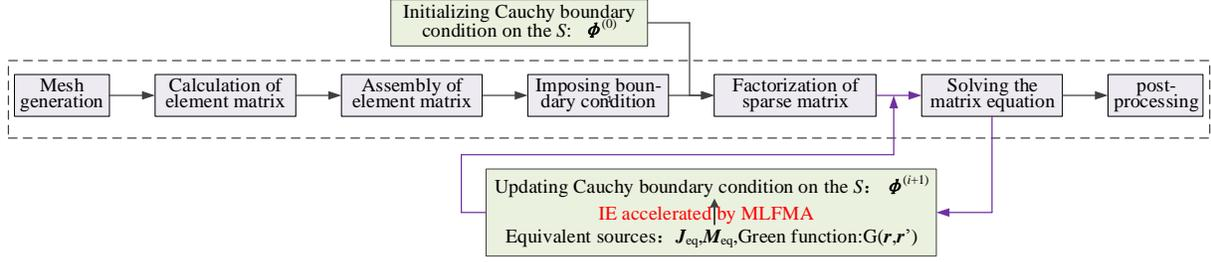
Fig. 3. The program design flow of the FE-IIIEE+MLFMA implemented in this paper.
