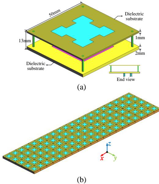
Fig. 10. The array antenna model: (a) the array unit structure, and (b) the array structure.
