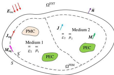
Fig. 1. A typical FE-IIIEE method for general radiation or scattering problems.
