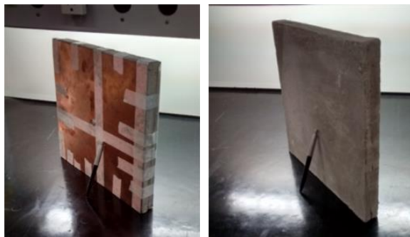
Fig. 4. (Left) Capacitor with its metallic plates and (right) its dielectric inner part.
