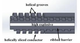
Fig. 14. Cross section of the ribbed barrier with helical grooves.
