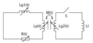
Fig. 7. Electrical circuit of cascaded-HFCG considering added resistance and dynamic  $L_p$ .
