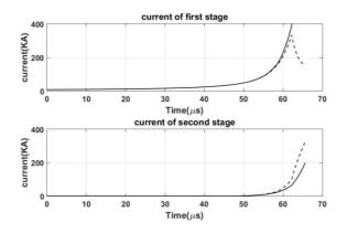
Fig. 8. Simulation results of conventional generator (solid line) and generator with time-varying  $L_P$  and incremental resistance (dashed line).
