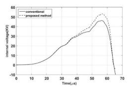
Fig. 9. Internal voltage for conventional generator (continued line) and proposed method (dashed line).
