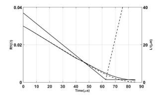
Fig. 6. Self-inductance and resistance profile of firststage winding; (solid line) conventional generator; (dashed line) generator with added resistance and timevarying L<sub>P</sub>.
