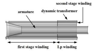
Fig. 3. FEM model of Cascaded-HFCG used to calculate inductances.
