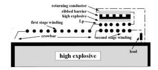
Fig. 13. Cascaded-HFCG with incremental resistance and time-varying  $L_P$ .
