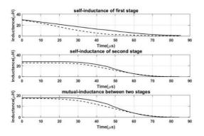
Fig. 5. Calculated time-varying inductances: (solid line) for FEM method; (dashed line) for 2-D filamentary method.
