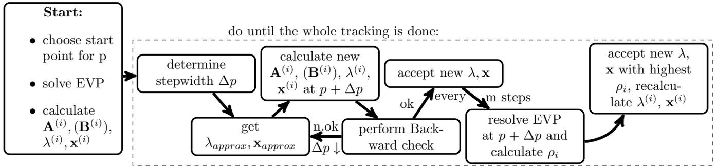
Fig. 1. Flowchart of the mode tracking algorithm.
