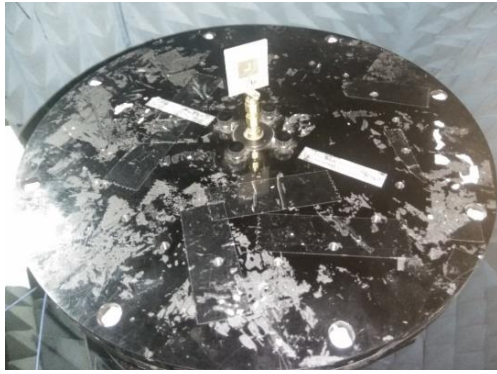
Fig. 8. Antenna mounted in anechoic chamber.
