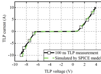
Fig. 7. TVS diode SPICE model simulation TLP results.
