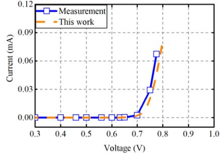
Fig. 5. Simulated and measured forward DC I-V curves.
