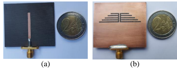
Fig. 2. Fabricated prototype of the proposed planar printed slot antenna: (a) top side and (b) bottom side.
