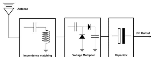
Fig. 1. General architecture of RF energy harvesting system.
