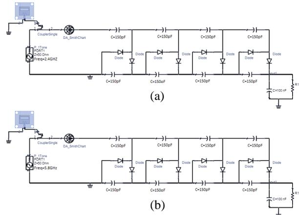
Fig. 4. Schematic diagram of 4-stage RF energy harvesting system for: (a) 2.4 GHz and (b) 5.8 GHz.
