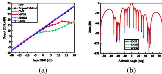
Fig. 3. (a) Output SINR versus the input SNR when parameter  $\varepsilon$  is equal to  $6 \times 10^{-10}$ , and (b) beam patterns of the proposed method when the number of snapshot takes different values and  $\varepsilon$  is equal to  $6 \times 10^{-6}$ .
