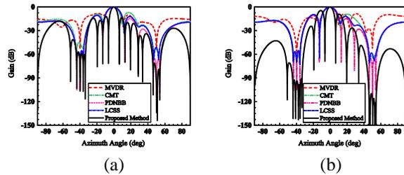
Fig. 2. (a) Normalized beampatterns of different algorithms when parameter  $\varepsilon$  is equal to  $6 \times 10^{-6}$ , and (b) normalized beampatterns of different algorithms when parameter  $\varepsilon$  is equal to  $6 \times 10^{-10}$ .
