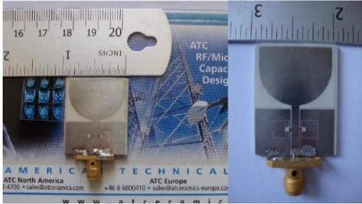
Fig. 2. Fabricated picture of the narrowband antenna.
