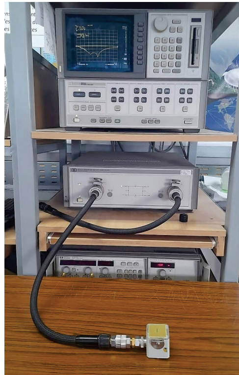
Fig. 12. Photograph of measurement set-up: Reflection coefficient measurement.
