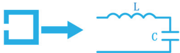
Fig. 4. Equivalent LC circuit of the SRR.
