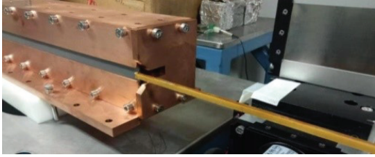
Fig. 9. Point coil for measuring the end field.
