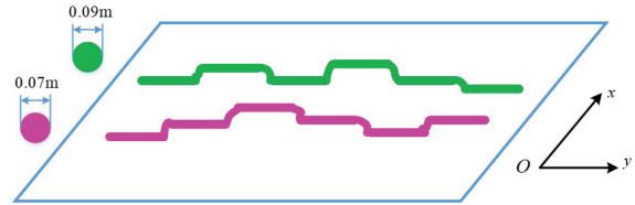
Fig. 2. Schematic diagram of the cable cascade model. The pink cable has electromagnetic interference, while the green one is the disturbed cable.
