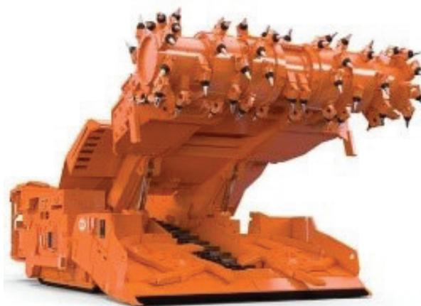
Fig. 1. Picture of a continuous miner commonly used in mining of coal, trona, salt and soft rock types. Pick cutters are mounted on a drum to apply force and break the rock [14].
