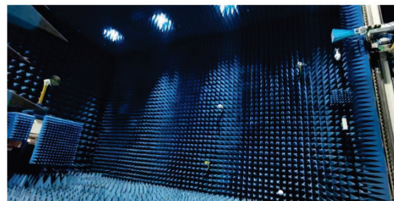
Fig. 12. Far-field measurement setup.
