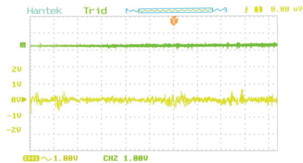
Fig. 17. Interference waveform of the LCD screen after adding suppression measures.
