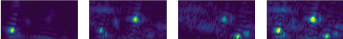
Fig. 3. Reconstructions of torso and arm cross section for three focusing cases and their combination: (a) focus on left arm, (b) focus on middle of torso, (c) focus on right arm and (d) complex combination of three images.
