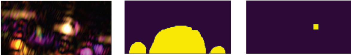
Fig. 4. The processed radar image of Fig. 2 along with its corresponding masks fed into the deep learning model for training: (a) RGB image, (b) body mask, (c) anomaly mask.
